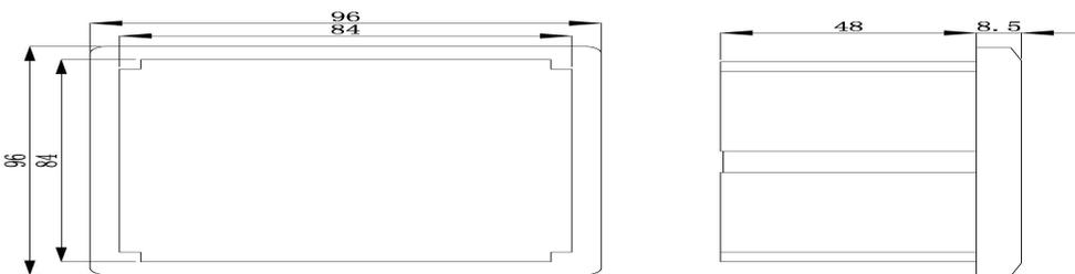
Size of form: 96 mm (Width) ×96 mm (Height) ×8.5 mm (Depth) (front panel)
